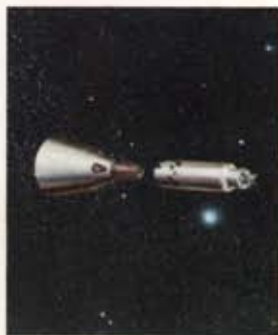
8. Vehicles make contact (at nearly identical orbital velocities) and are latched together.
