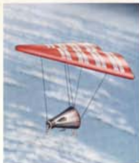
12. Paraglider deployment is complete at 40,000 feet.
