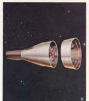
10. After unlatching, Gemini equipment section is jettisoned.
